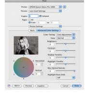
Epson's "Advanced Black and White Photo Mode" utilizes the three-level UltraChrome K3 Ink black and gray inks to provide excellent neutrality throughout the tonal scale and also allows the user to shift the overall hue or "tone" of a monochrome image.
